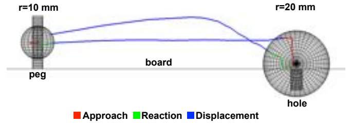
Fig. 5. Front view of the decomposition of one trajectory into approach, reaction and displacement phases based on a spherical area around the peg ( r=10 mm, centered on the middle of a peg at its initial position) and around the hole ( r=20 mm, centered on the middle of a peg when inserted in the hole).
